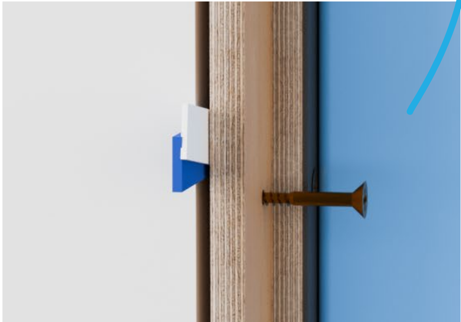
Place packers above or behind fixings ensuring the frame is pushed away from the opening for fire-stopping material to be added.
