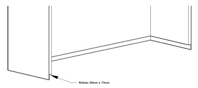
2. Fix the plinth to the floor and wall using the brackets supplied, ensuring that the top of the plinth is level (if multiple Hygipods are being installed, continuous plinth may be supplied, to be cut to length on site).
