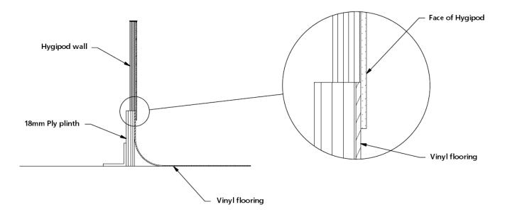
3. If vinyl flooring is to be coved to the plinth, this should be installed at this stage.
