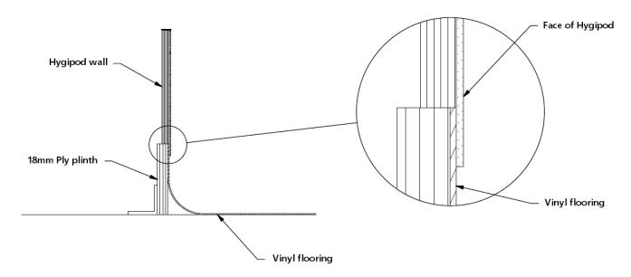
3. If vinyl flooring is to be coved to the plinth, this should be installed at this stage.
