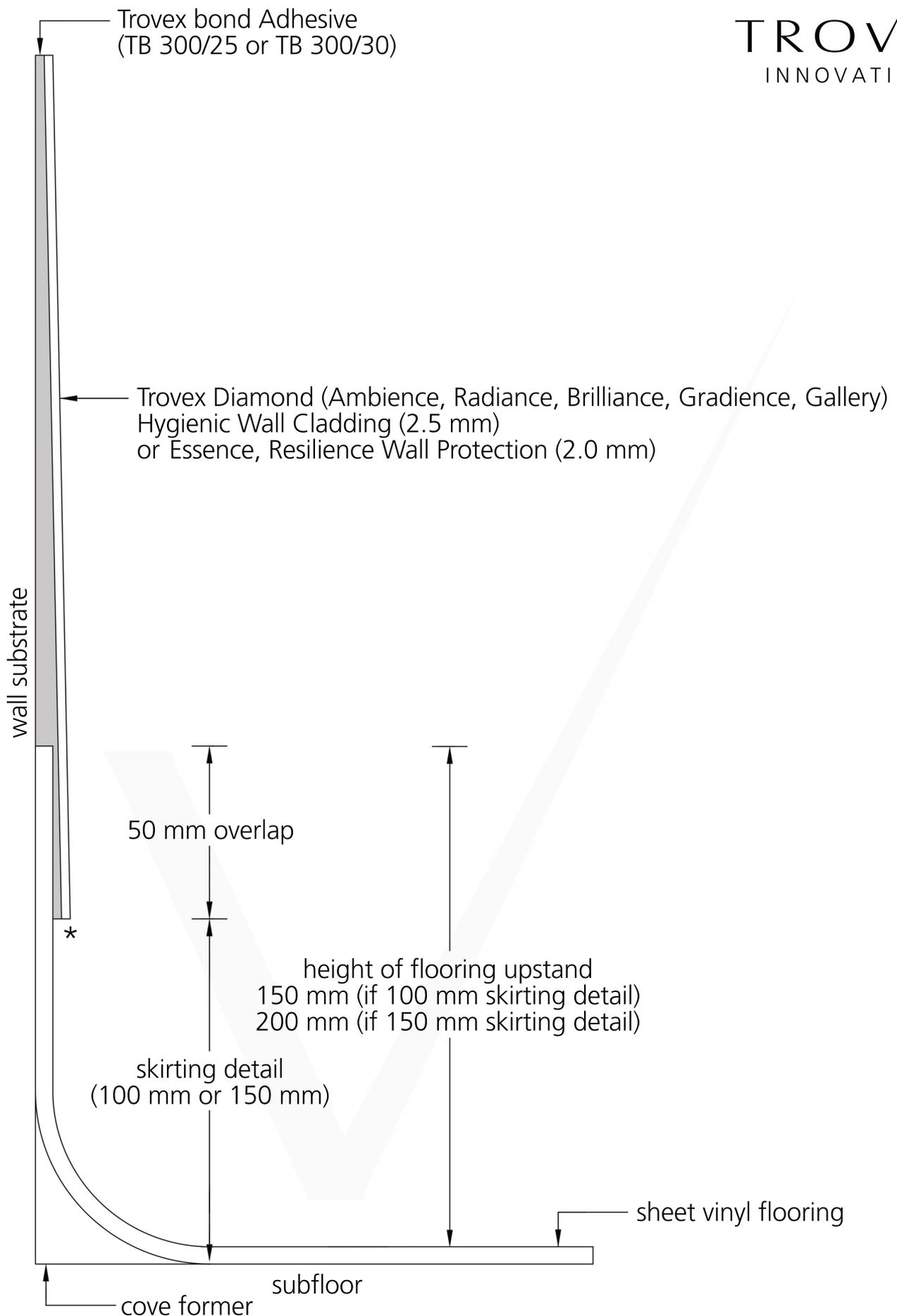
\* can be sealed with silicon sealant or anti-pick mastic if required
