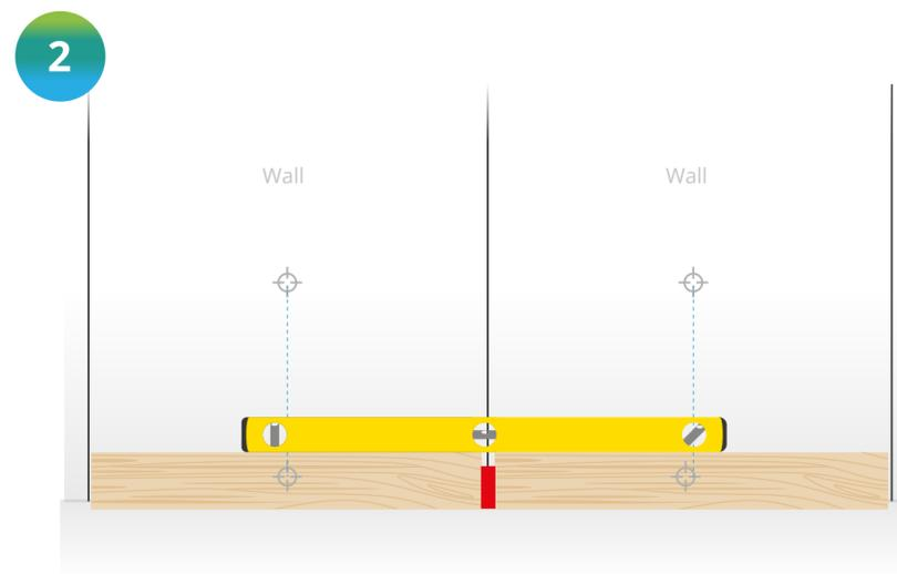
2 Position the first plinth centred to the first set of markings, then place a 15mm packer between the subsequent plinth.
