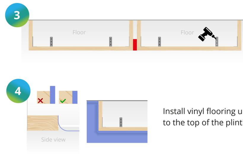
3 Fix the plinths to the floor and wall using the supplied brackets.
