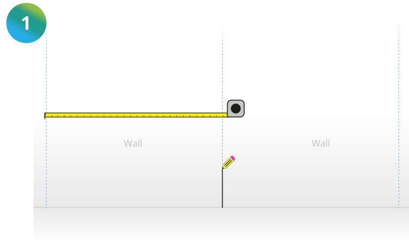
1 Determine the location of the Hygipods and accurately mark the width of the units onto the wall.
