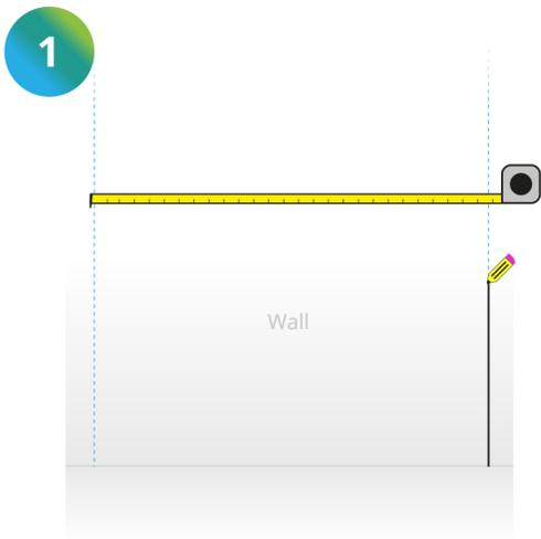
1 Determine the location of the Hygipod and accurately mark the width of the unit onto the wall.
