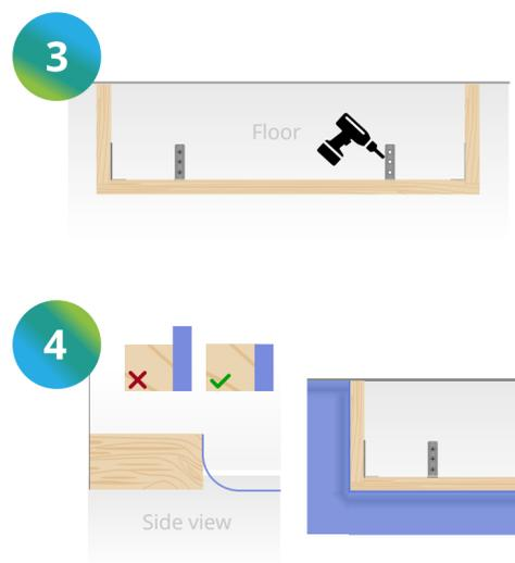
3 Fix the plinth to the floor and wall using the supplied brackets.
